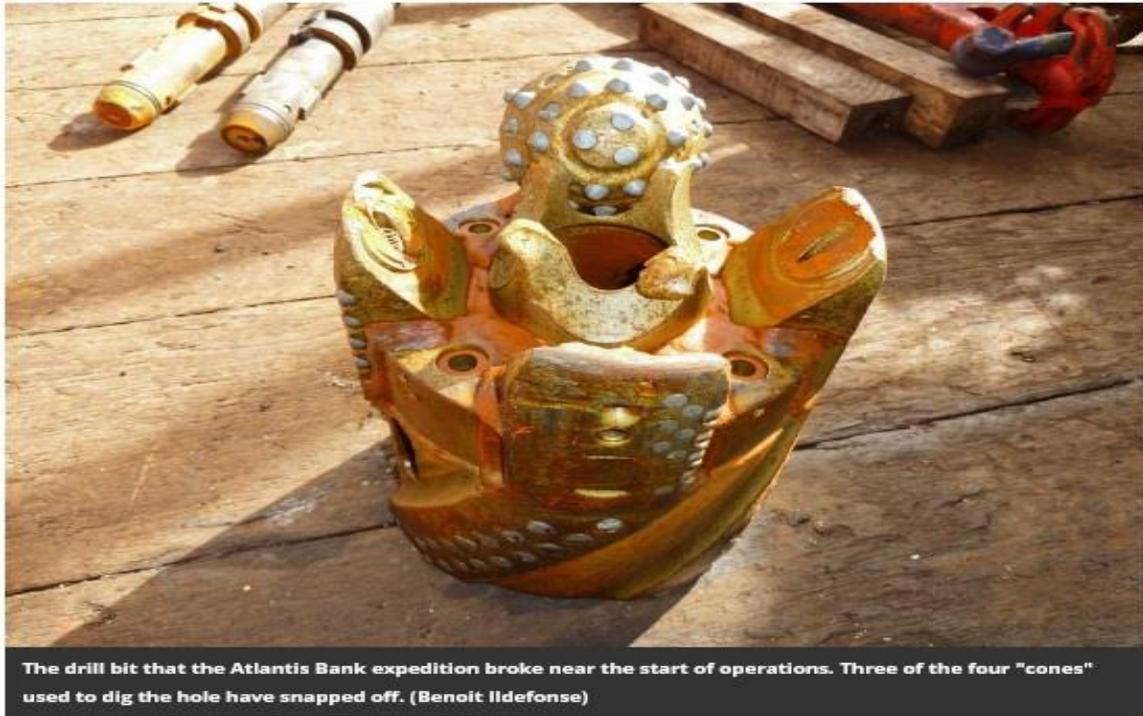
The drill bit that the Atlantis Bank expedition broke near the start of operations. Three of the four "cones" used to dig the hole have snapped off. (Benoit Ildefonse)
